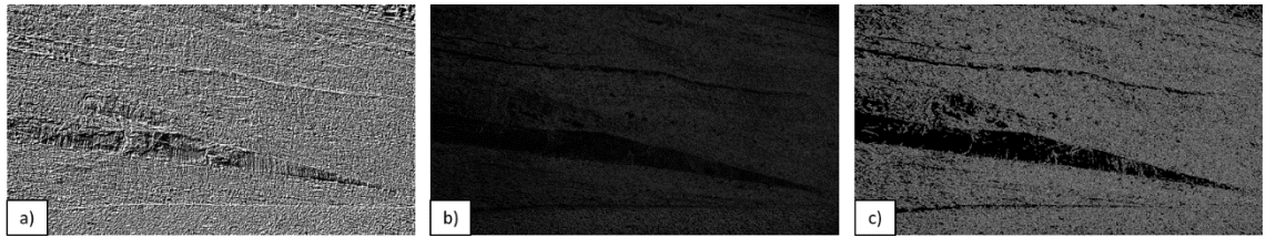
Figure 3-9: Unsupervised Segmentation Edge Detection techniques, including a) Sobel, b) LoG, and c) Canny Edge detection.
