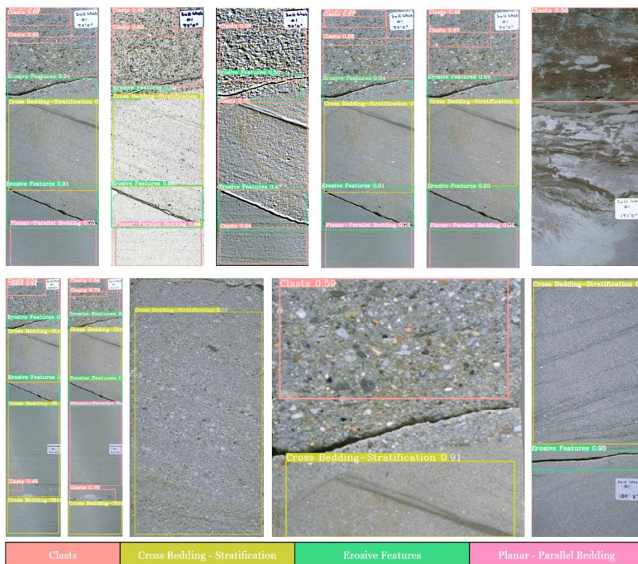
Figure 6-19: Results of the application of the YOLOv6-S model on the distorted images of core samples.
